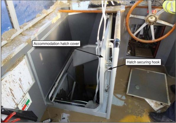
Figure 4: Accommodation hatch cover (hooked open)
