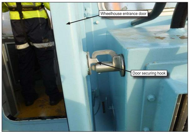
Figure 5: Wheelhouse entrance door (hooked open)
