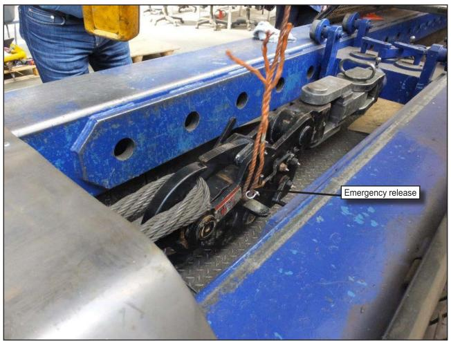
Figure 13: Towing hook emergency release testing
