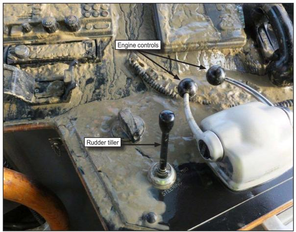
Figure 6: Asterix manoeuvring controls
