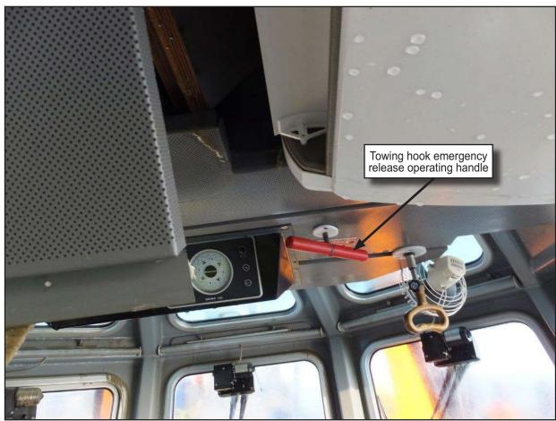
Figure 8: Towing hook emergency release handle
