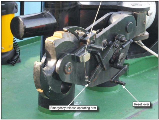
Figure 10: Towing hook emergency release arrangement
