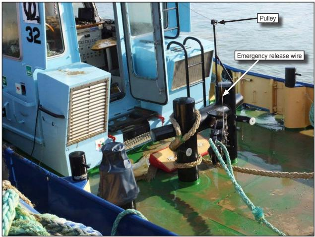
Figure 9: Towing hook emergency release wire
