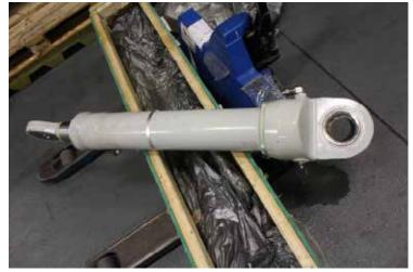
Figure 6 Wing landing gear actuator
