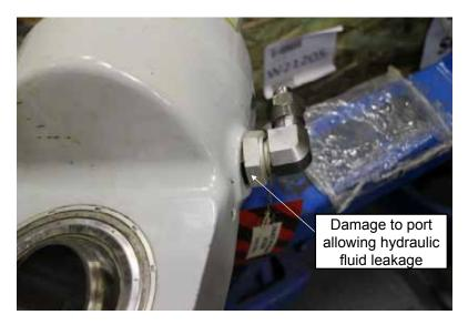
Figure 3 Damaged hydraulic port on landing gear actuator
