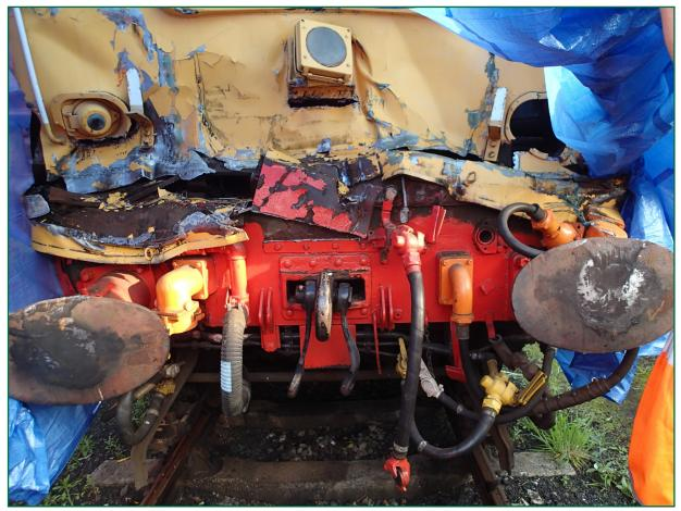
Figure 10: Damage sustained by locomotive 37198 following the collision
