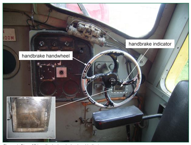
Figure 4: Class 37 handbrake hand wheel and indicator
