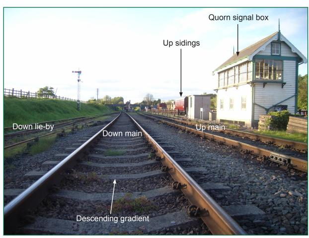
Figure 2: Layout of the track opposite Quorn signal box.
