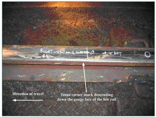
Figure 7: Tread corner marks descending down the gauge face of the right hand rail head
