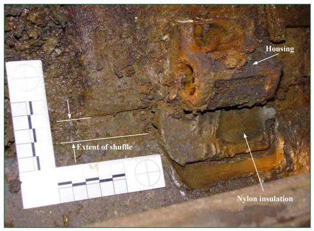
Figure 4: Sleeper 105 showing the degree of rail shuffle that had taken place (note the missing Pandrol clip)
