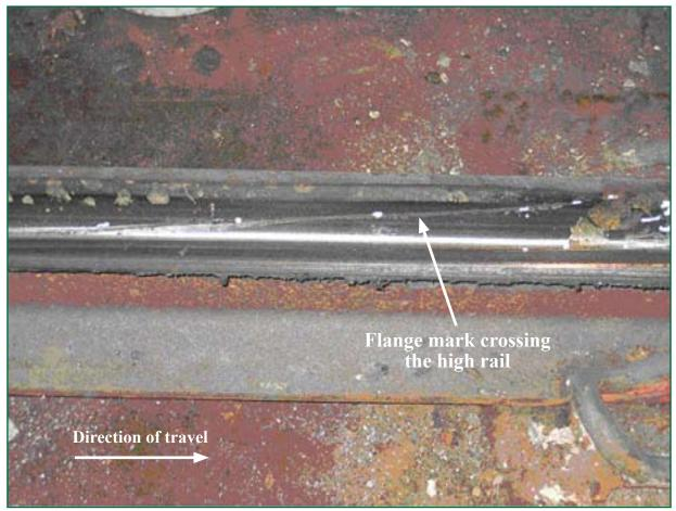
Figure 9: Flange climb mark up the gauge face of the high rail between the second and third sleepers
