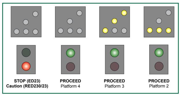
Figure 13: Routes applicable to the arbour lights junction indicators on signals ED23 and RED230/23 (Note: when at Caution, RED230/23 shows a yellow lower aspect)
