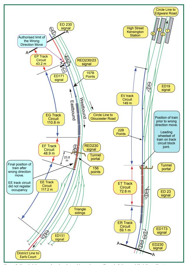
Figure 3: Detailed diagram of track and signal layout between Triangle Sidings and High Street Kensington
