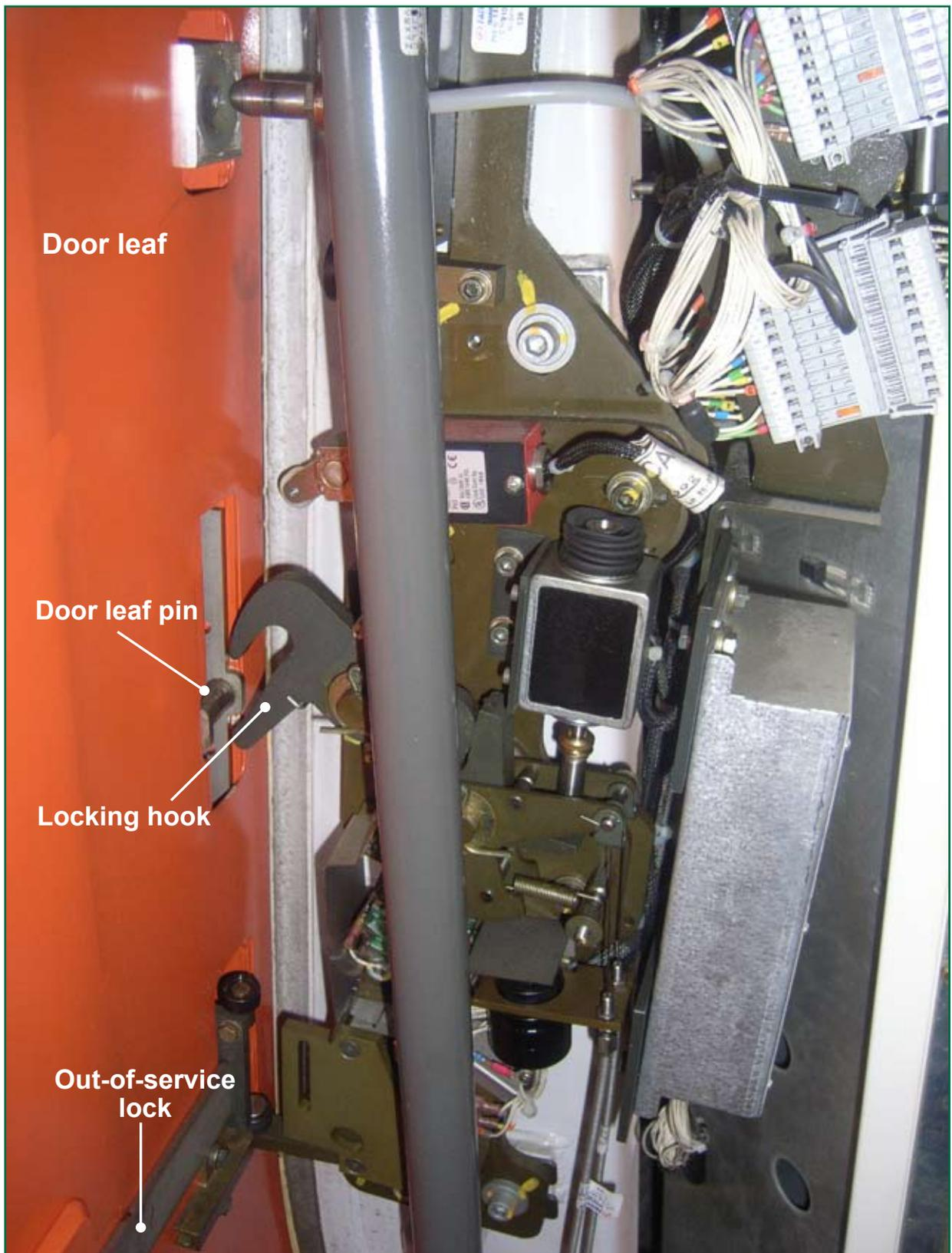
Figure 7: Door lock assembly showing its relationship to the door leaf (shown with door unlocked and unplugged)
