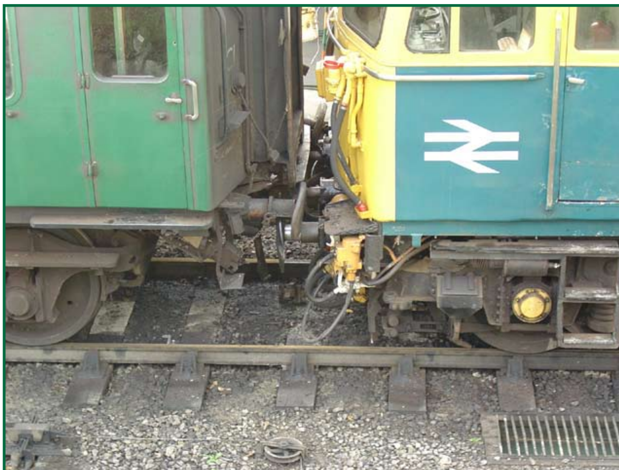
Figure 2: Damage sustained to the locomotive and carriage
