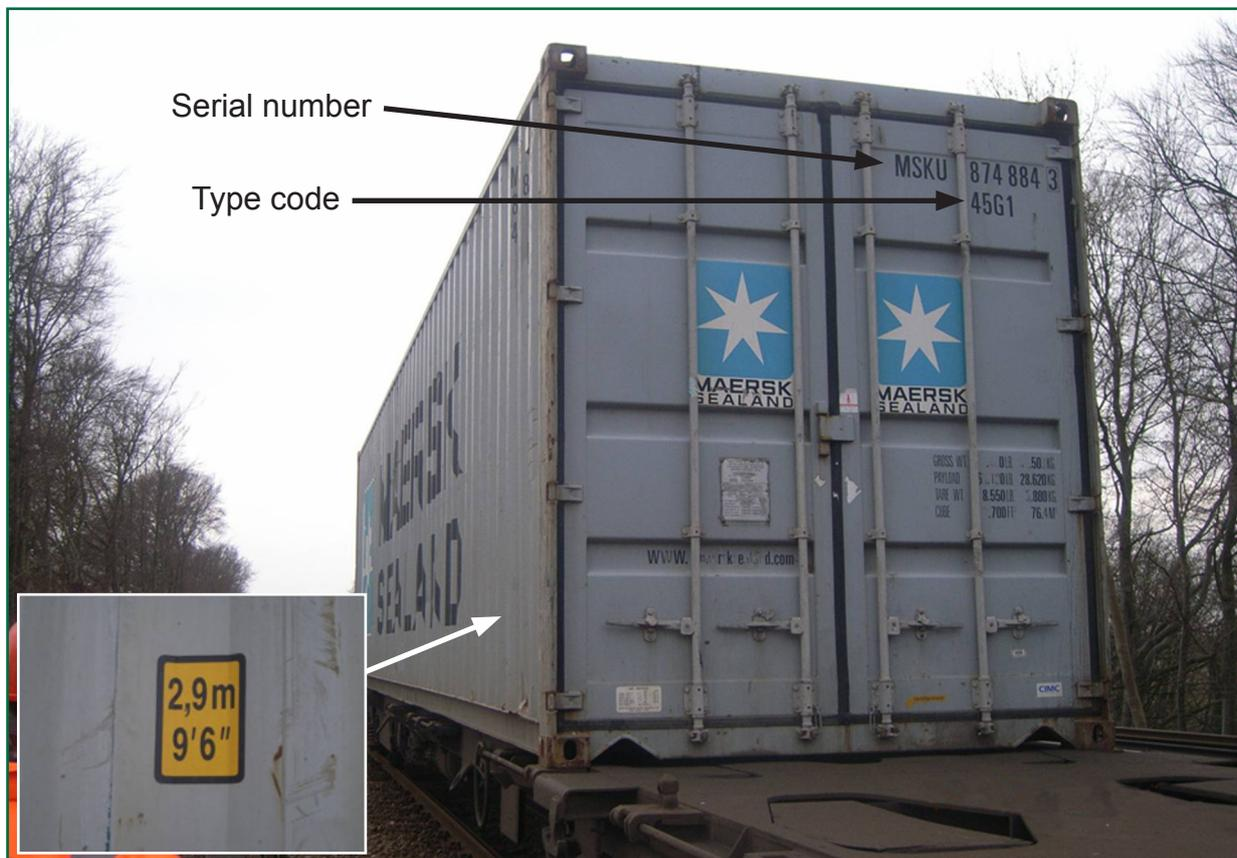
Figure 9: Incident container showing serial number, type code, position of height marking (on sides), and absence of black/yellow stripes
