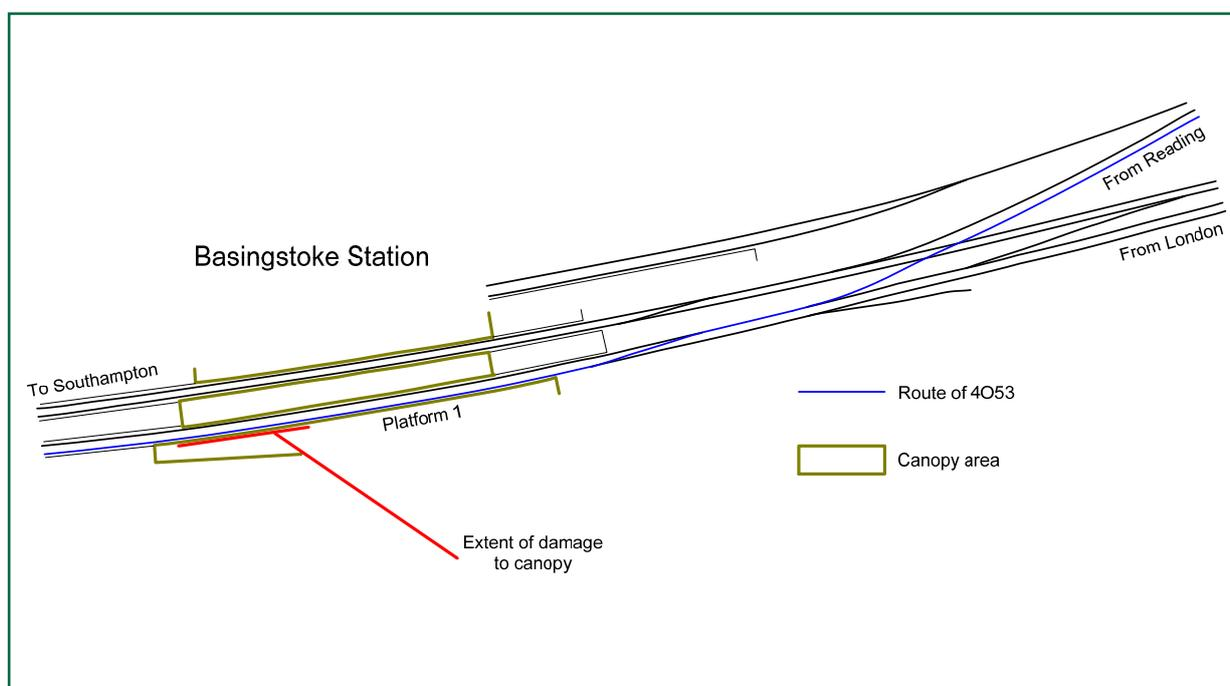
Figure 3: Basingstoke station showing route of train
