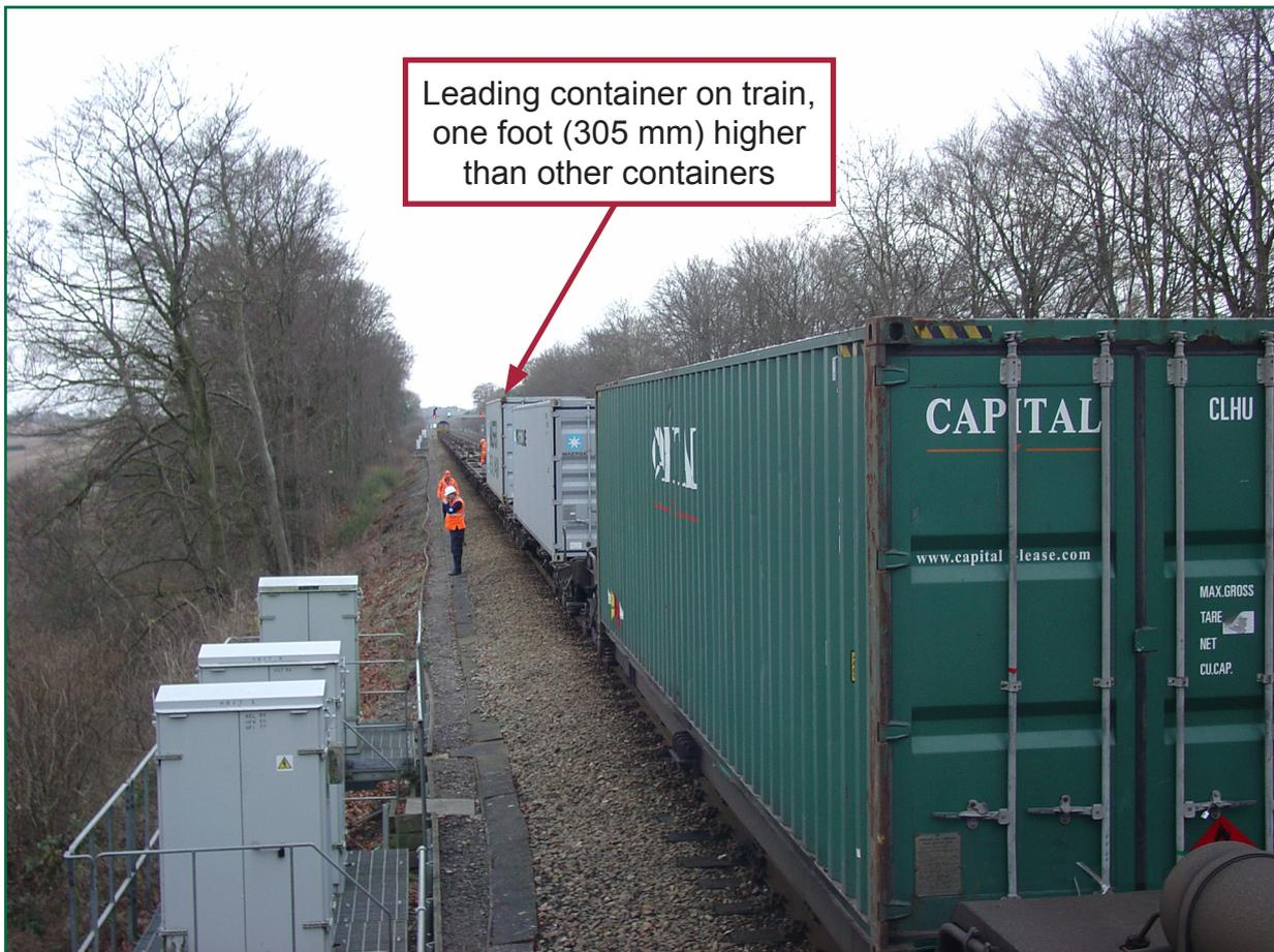
Figure 7: Train at Waller's Ash loop, showing overheight container
