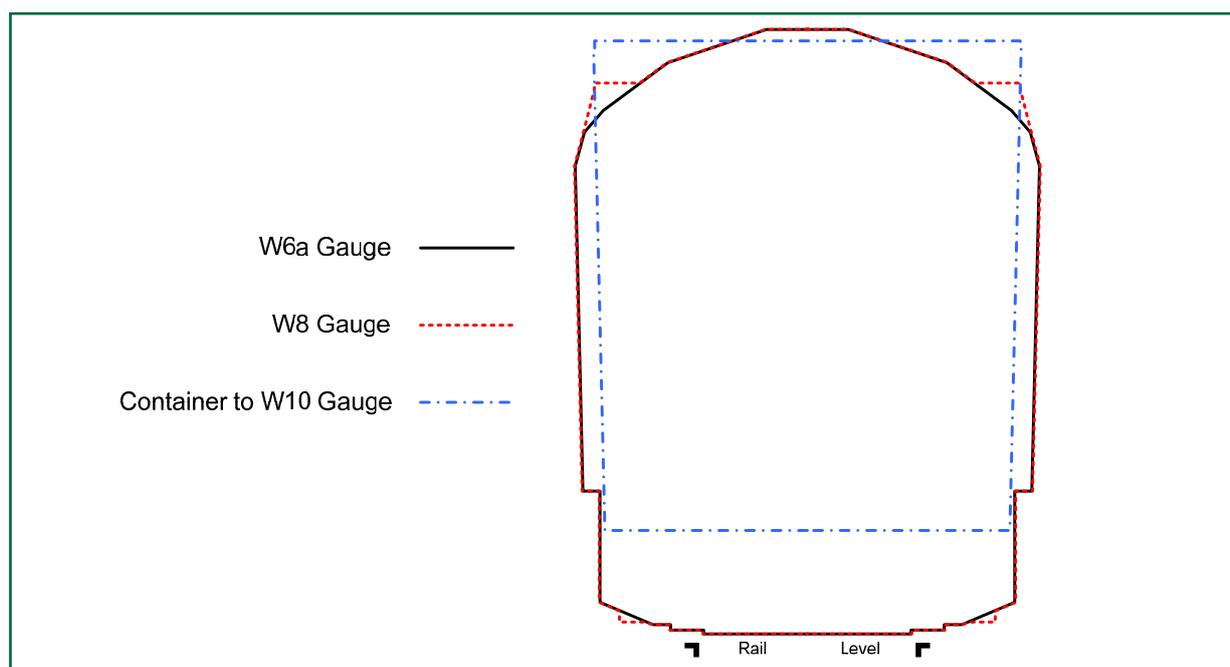
Figure 8: Standard vehicle gauges (incorporating dynamic movements)
