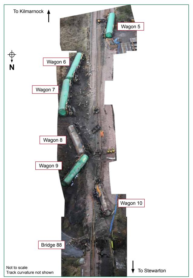
Figure 2: Composite aerial photograph showing the collapsed bridge and the location of the derailed wagons on the southern side (photographs courtesy of Network Rail)
