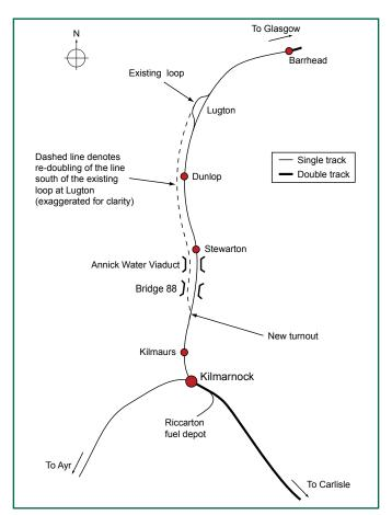
*Figure 3: Diagram of the railway between Barrhead and Kilmarnock (not to scale)*
