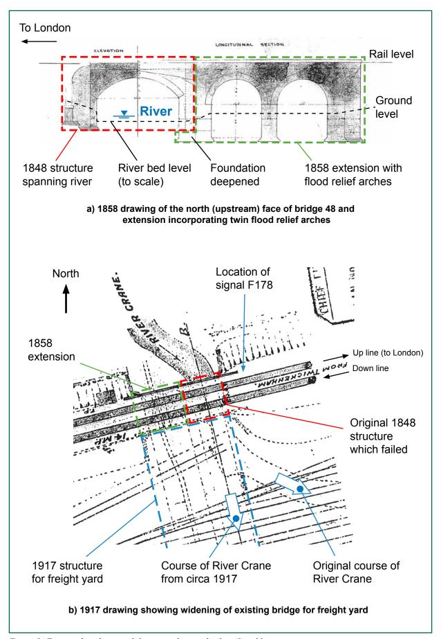
Figure 3: Extracts from historical drawings showing bridge 48 and later extensions
