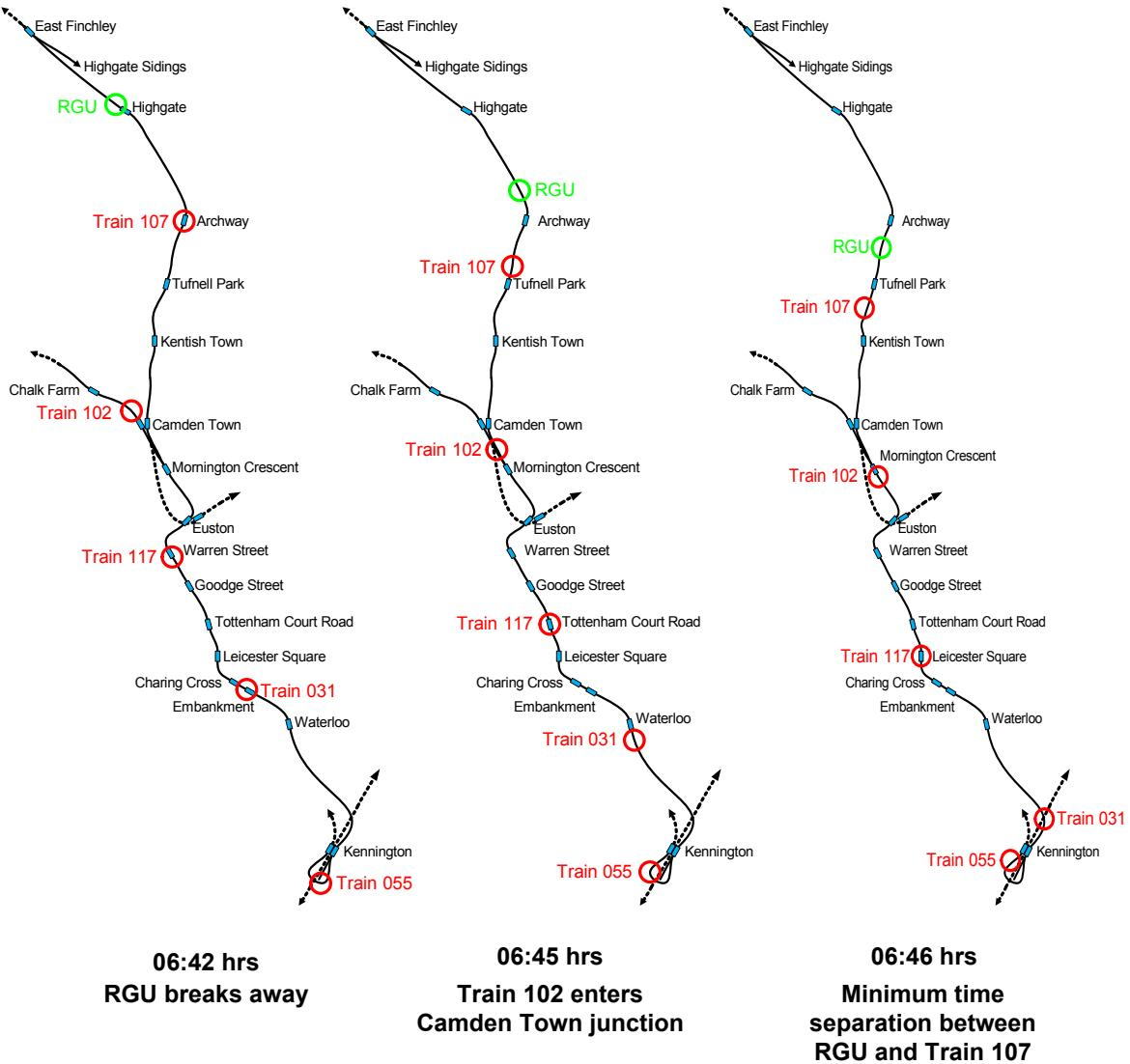
Figure 8: Train positions during the runaway.
