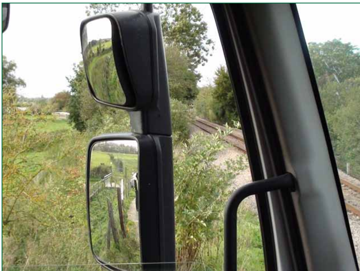
Figure 8: View of train taken from the tanker vehicle driving position showing the train beyond Shalfords UWC at around 500 metres (Photograph from the sighting tests on 3 October 2010)
