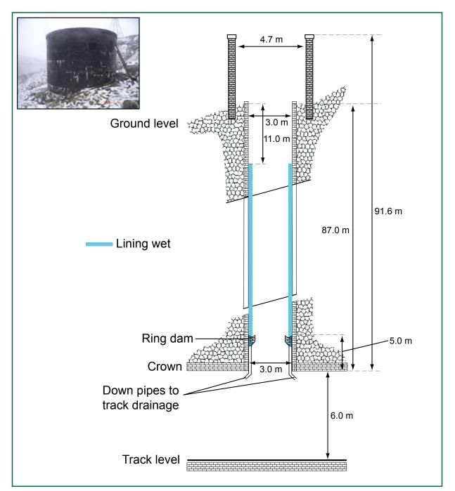
Figure 14: Diagram showing dimensions and key features for ventilation shaft 10
