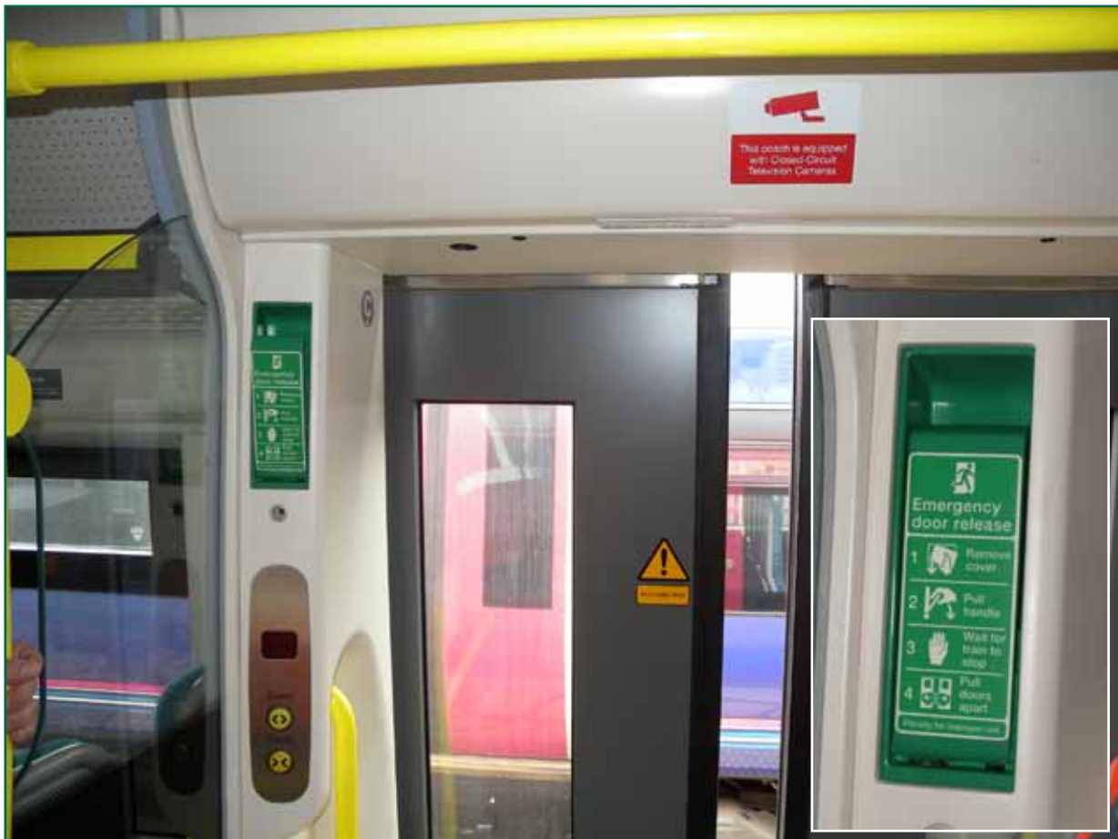
Figure 9: Door egress handle allowing partial opening of the train door after egress handle is pulled down (inset - egress alarm in its normal state)
