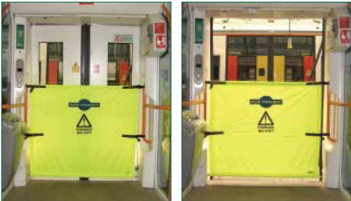
Figure 13: Emergency door screen equipment (images courtesy of FCC and Southern Railways)
