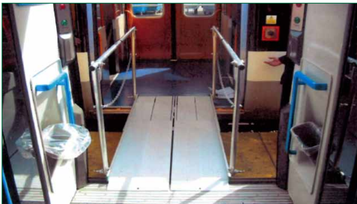
Figure 12: Transboardment bridge (image courtesy of Southeastern, the developers of the bridge)
