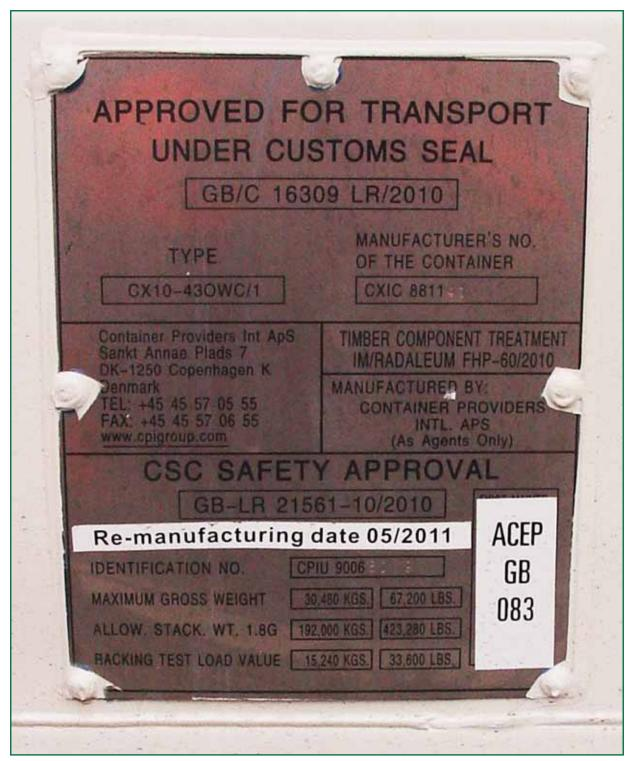
Figure 10: Safety approval plate fixed to container CPIU 9006609. The RAIB understand that the white decal, entitled 'Re-manufacturing date 05/2011', was affixed when the container was modified (paragraph 20). Note: Recognised by the CSC as acceptable practice, the safety approval plate has been grouped with other official plates on one base plate
