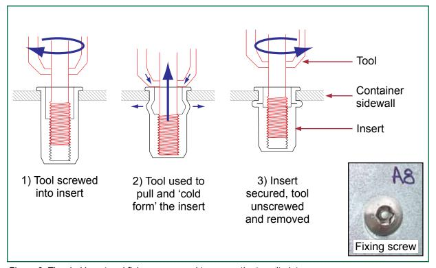
Figure 6: Threded insert and fixing screw used to secure the transit plate
