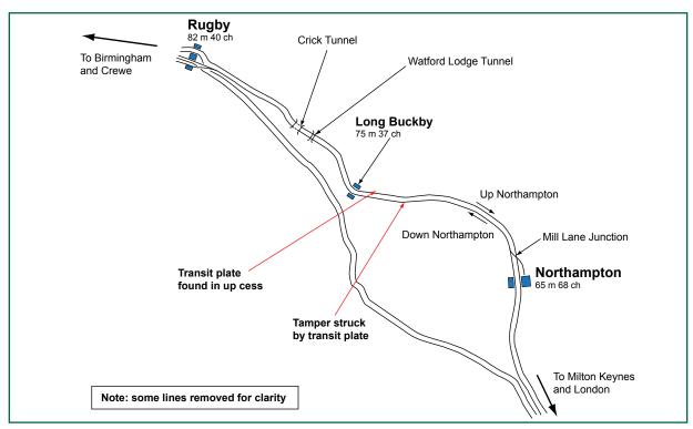
Figure 2: Diagram of the railway between Rugby and Northampton
