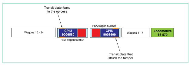
Figure 3: Configuration of train 4L68
