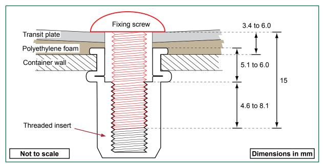
Figure 12: Cross-section through a typical bolted joint used on CPIU 9006609
