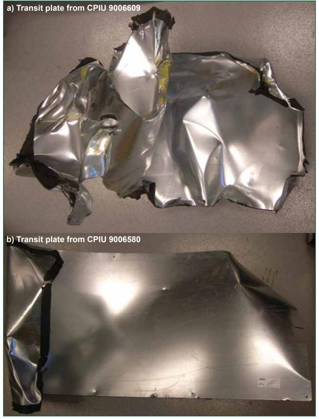
Figure 11: The transit plates that detached from containers CPIU 9006580 and 9006609 on train 4L68
