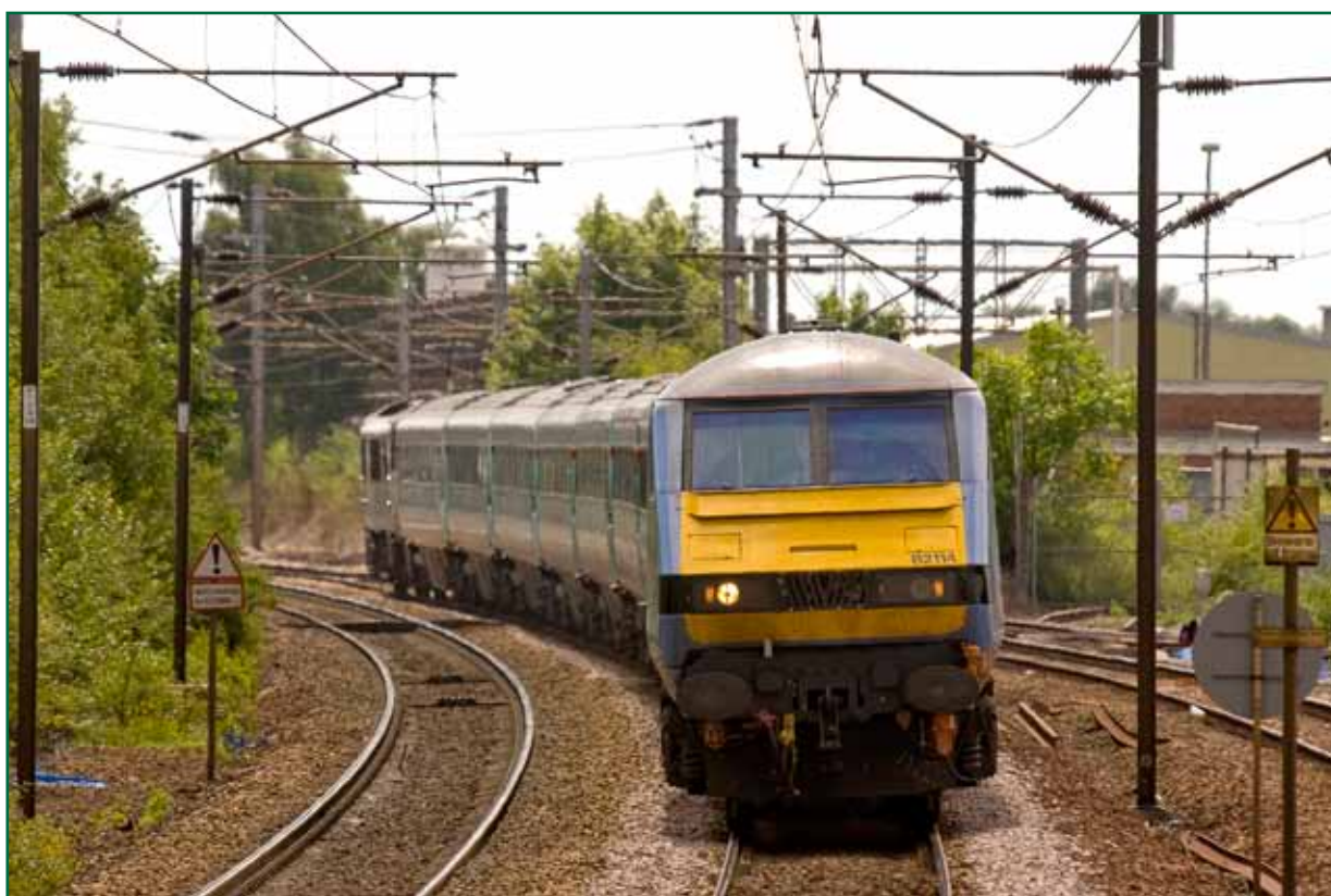
Figure 4: A DVT leading a train formed of Mark 3 coaching stock. A class 90 locomotive is attached at the rear of the formation (not the train involved or the location of accident) (image courtesy of Kev Gregory/Railway Herald)
