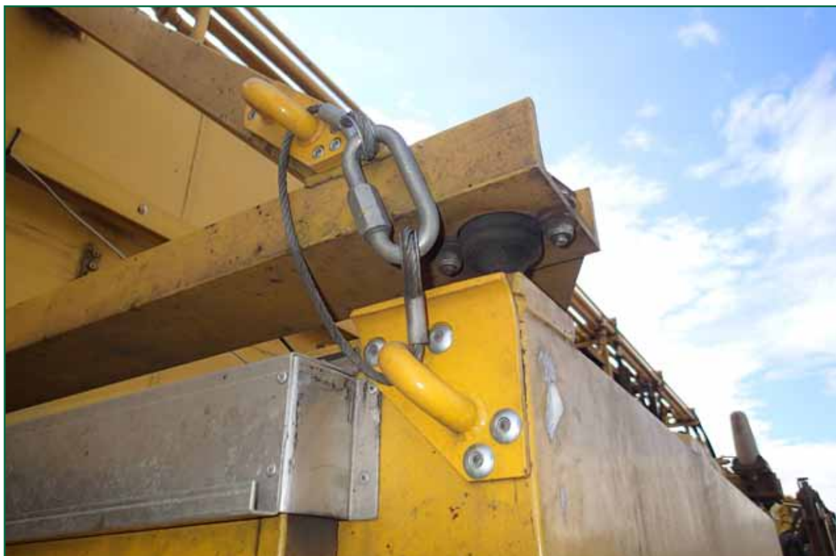
Figure 25: Secondary retention system fitted to each of the four corners of the P3 cab
