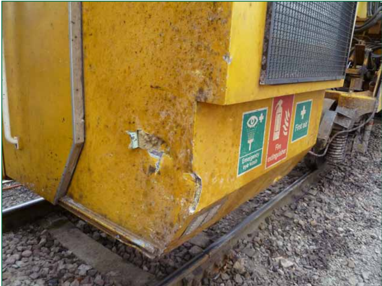
Figure 22: The damaged leading left edge of the P3 control cab following impact from the detached clamp on 26 January 2011
