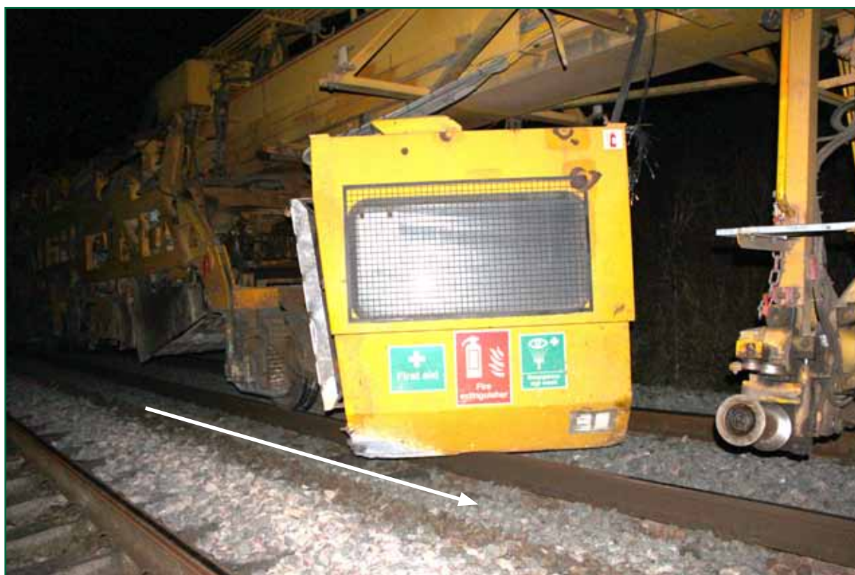
Figure 7: The detached control cab (path of train 6Y33 indicated by white arrow)
