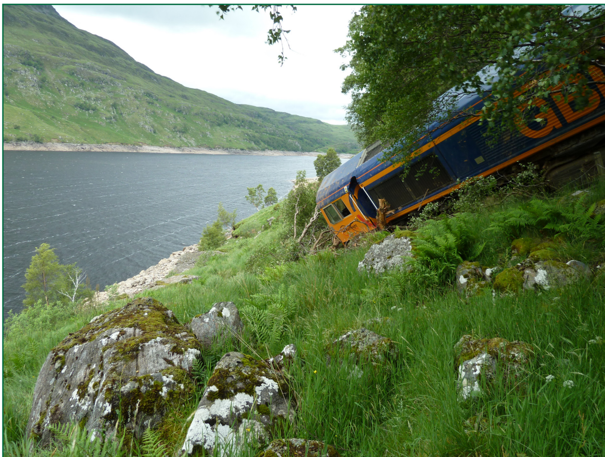
Figure 4: Loch Treig: derailed locomotive (image courtesy of Network Rail)
