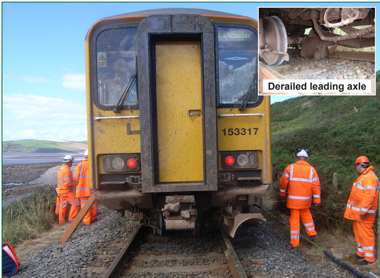
Figure 20: St Bees: derailed train
