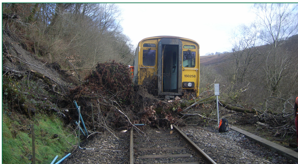
Figure 26: Bargoed: derailed train
