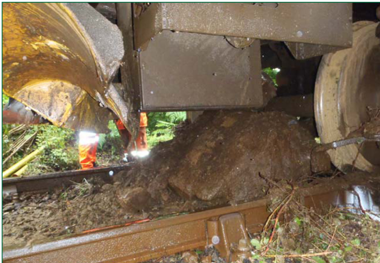
Figure 8: Falls of Cruachan: debris preventing train movement (image courtesy of Network Rail)
