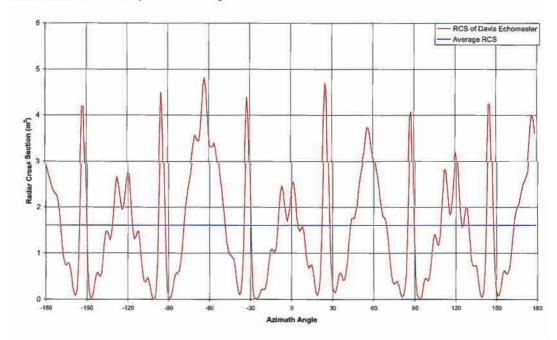
Figure 5 RCS plot of a Davis Echomaster radar reflector at X-Band.
