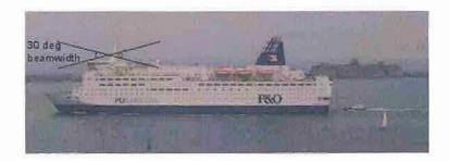
Figure 7 Diagram showing the elevation beamwidth of the S-Band radar overlaid on a photo of the Pride of Bilbao
