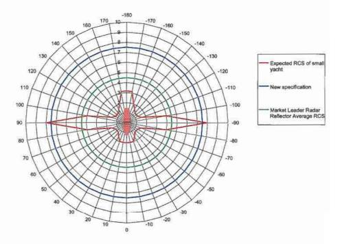
Figure 2 Plot showing expected RCS levels in m<sup>2</sup> against aspect angle for a yacht against expected returns from a radar reflector.
