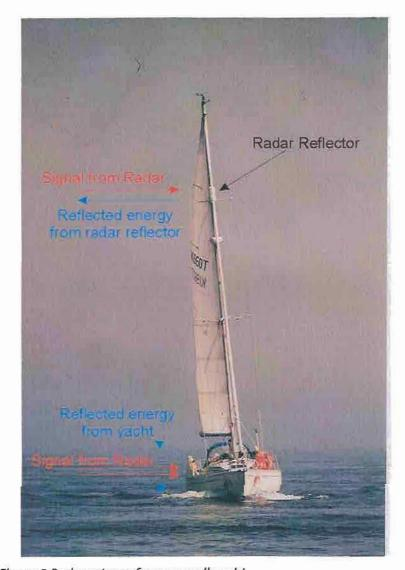
Figure 3 Radar returns from a small yacht
