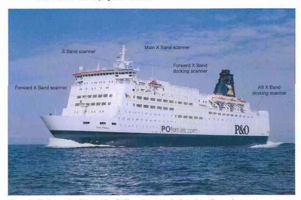
Figure 6 Photograph of the Pride of Bilbao showing the location of its radar scanners.
