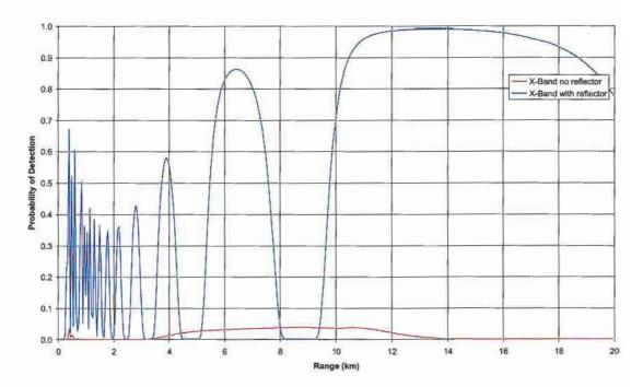
Figure 9 Probability of Pride of Bilbao's X-Band radar being able to detect a yacht with and without a radar reflector.
