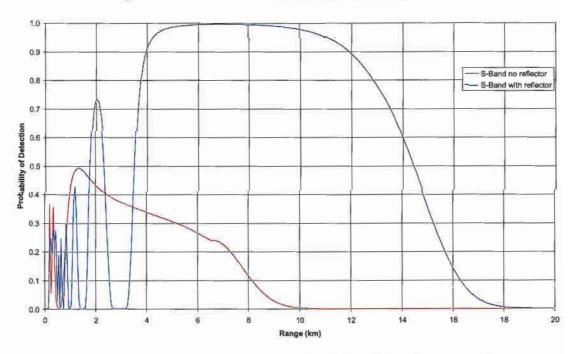
Figure 8 Probability of Pride of Bilbao's S-Band radar being able to detect a yacht with and without a radar reflector.
