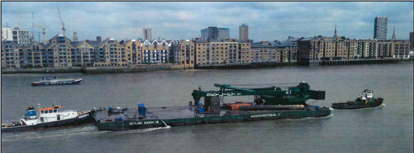
On 12 August 2011, the tugs *Steven B* and *Chiefton* were connected to a 60m crane barge in a combined push/pull configuration. *Steven B* was secured aft with a combination of wires and ropes, making the tug and barge a composite unit. The distance between *Chiefton*, which was pulling, and the barge was 8.4 metres. There were two pilots positioned on the crane as the tow was navigated from St George Wharf towards Gravesend on the River Thames.
