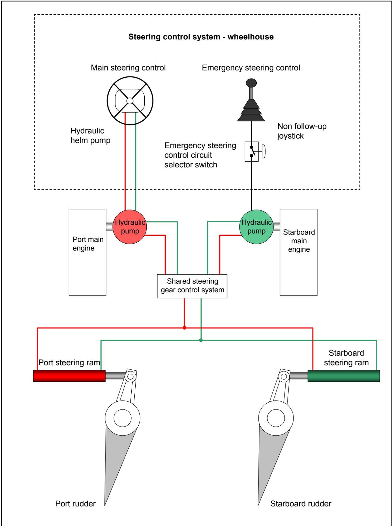
**Figure 15:** Simplified illustration of the steering gear control system
