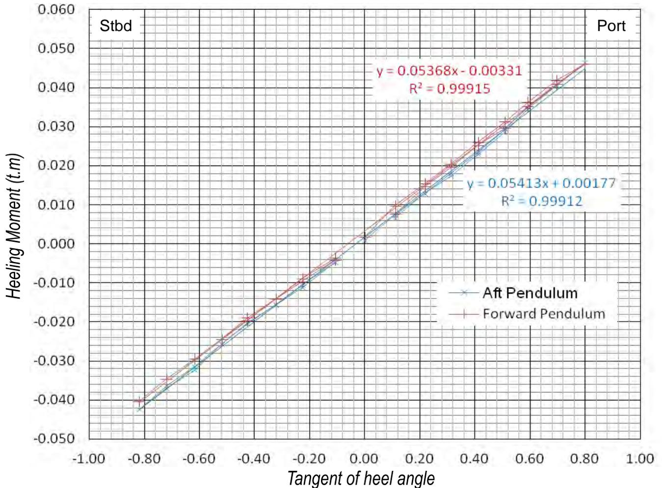
Mean slope (tangent) of aft pendulum = 0.05413 (correlation coefficient 0.99912)
