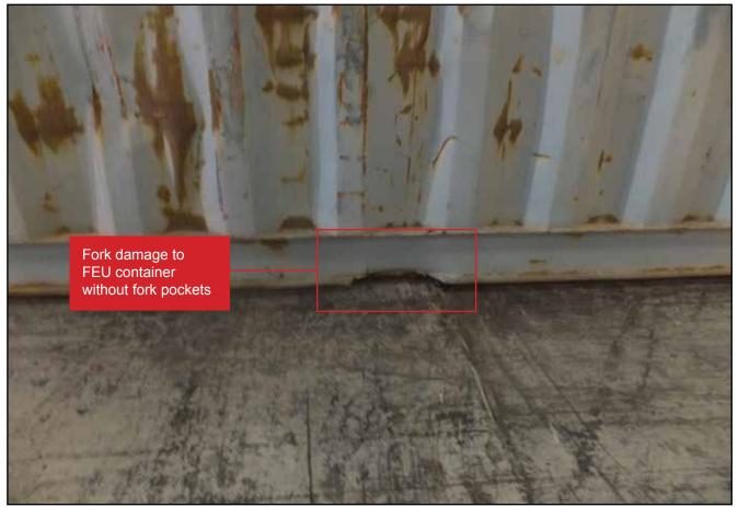
Figure 6: FEU container without fork pockets showing fork damage
