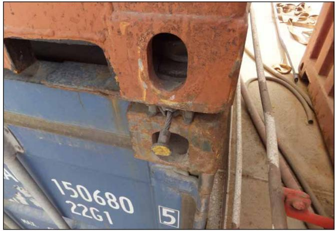
Figure 7: Semi-automatic twistlock securing two containers together
