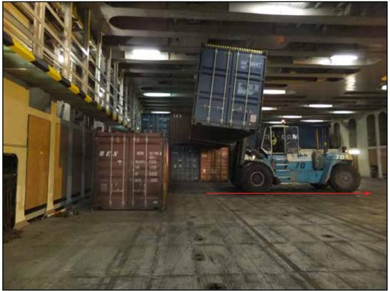
Figure 1d: Reconstruction – fork-lift truck reversing to move container A clear of container B
