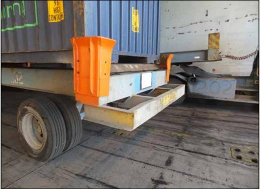
Figure 3: Trailer closed-corner and rear bumper fittings
