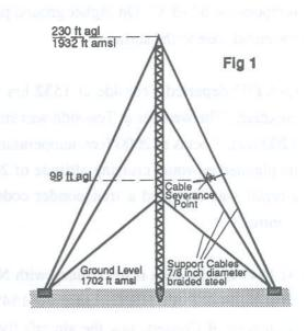
Three regions of the aircraft sustained cable strikes. This had caused detachment of the glass reinforced plastic tip of the left wing, the left aileron and the outboard four feet of the left wing; minor damage to the propeller; disruption of the right side of the forward fuselage; and gross damage at the right wing root that almost detached the right wing. Inaccessibility of the cables prevented full
