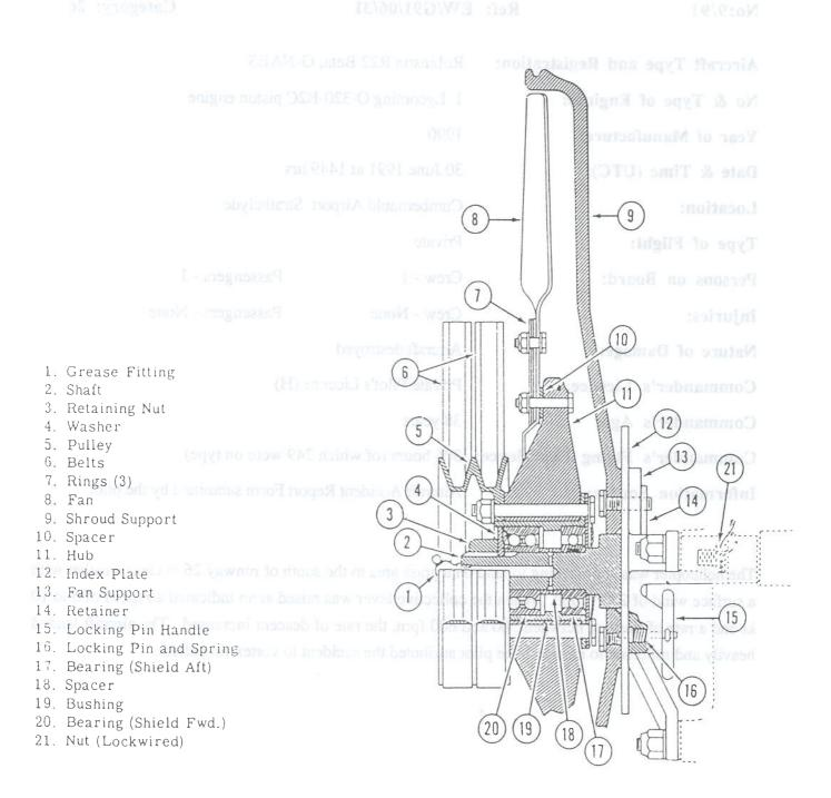
FIGURE 3 Diagram of Cooling Fan Assembly
