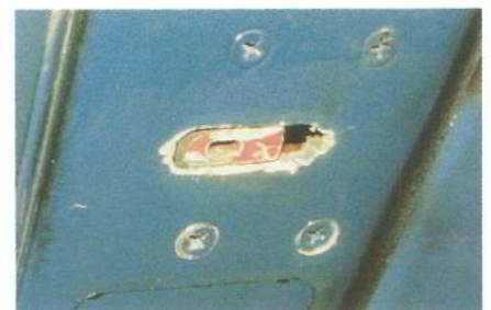
Visual Lock Indicator showing T/R closed and locked
