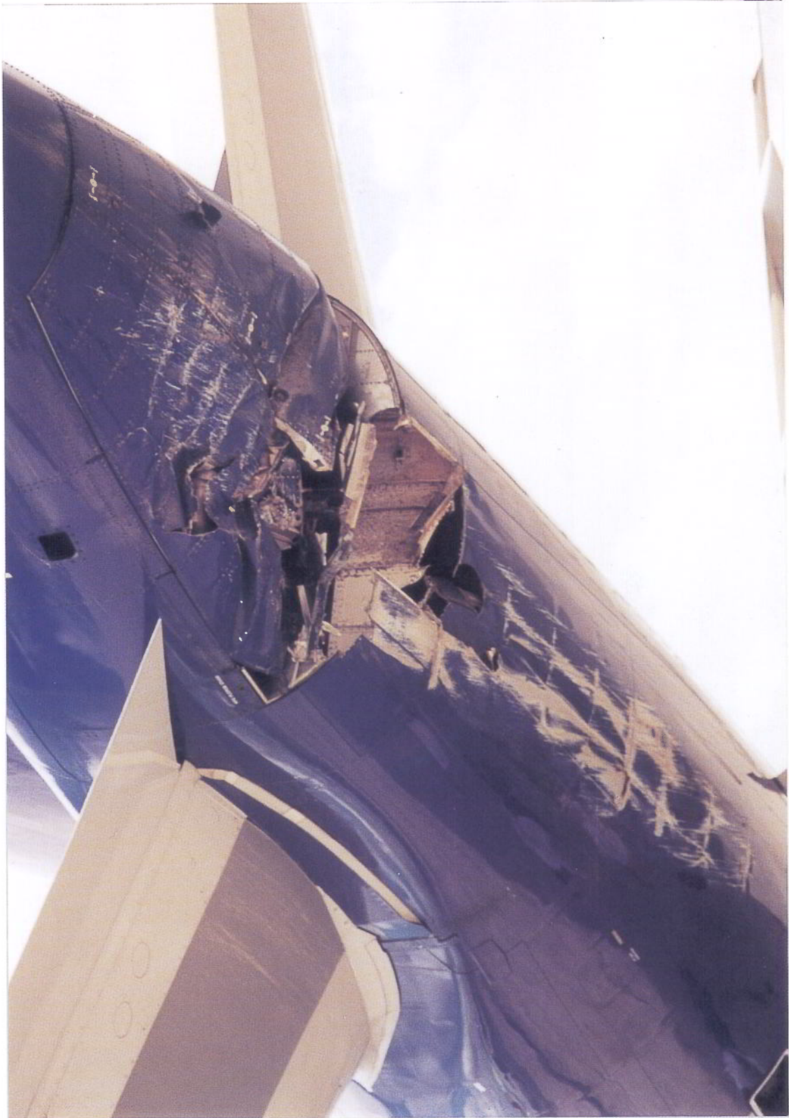
Figure 3 View of damage to rear fuselage
