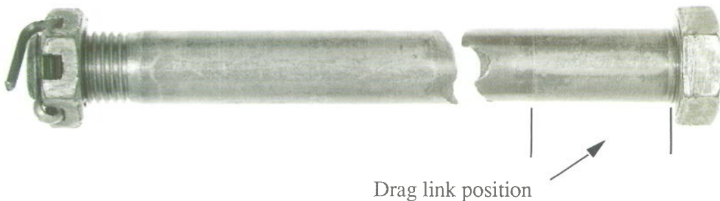
Failed drag link attachment bolt (Photo: DRA)
