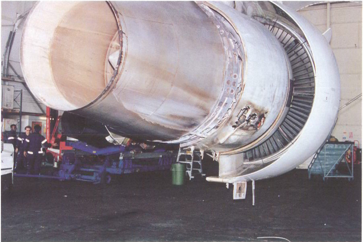
Fig.2. External view of No. 1 engine showing fire damage
