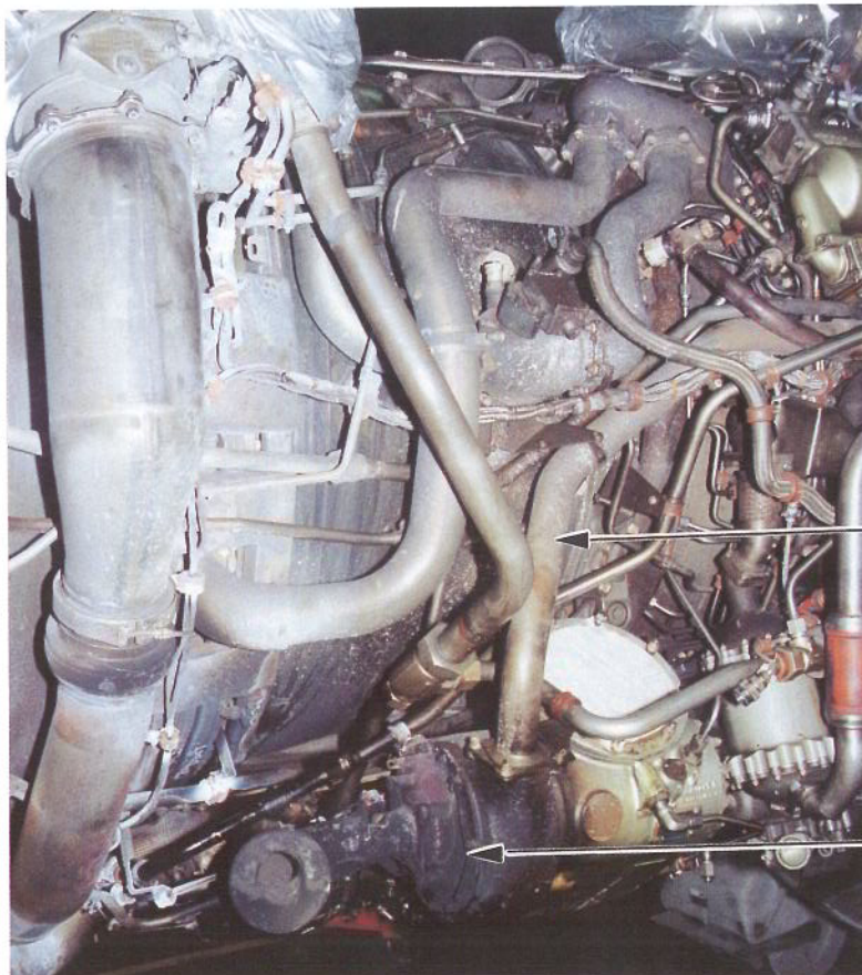
Fig.3. Right hand side of engine showing fire-damaged deaerator
