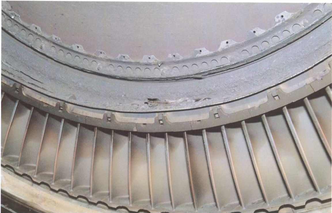
Fig.5. View looking aft onto damaged third stage NGV shroud
