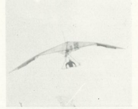
6. Apparent start of push on the control bar, indicated by change of body silhouette.
