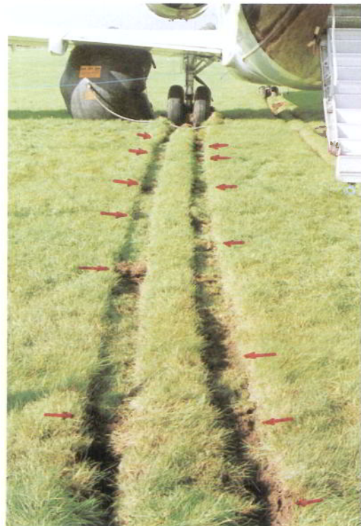
Left Main Tyre Tracks Across Stopway Arrows Indicate Skid Marks
