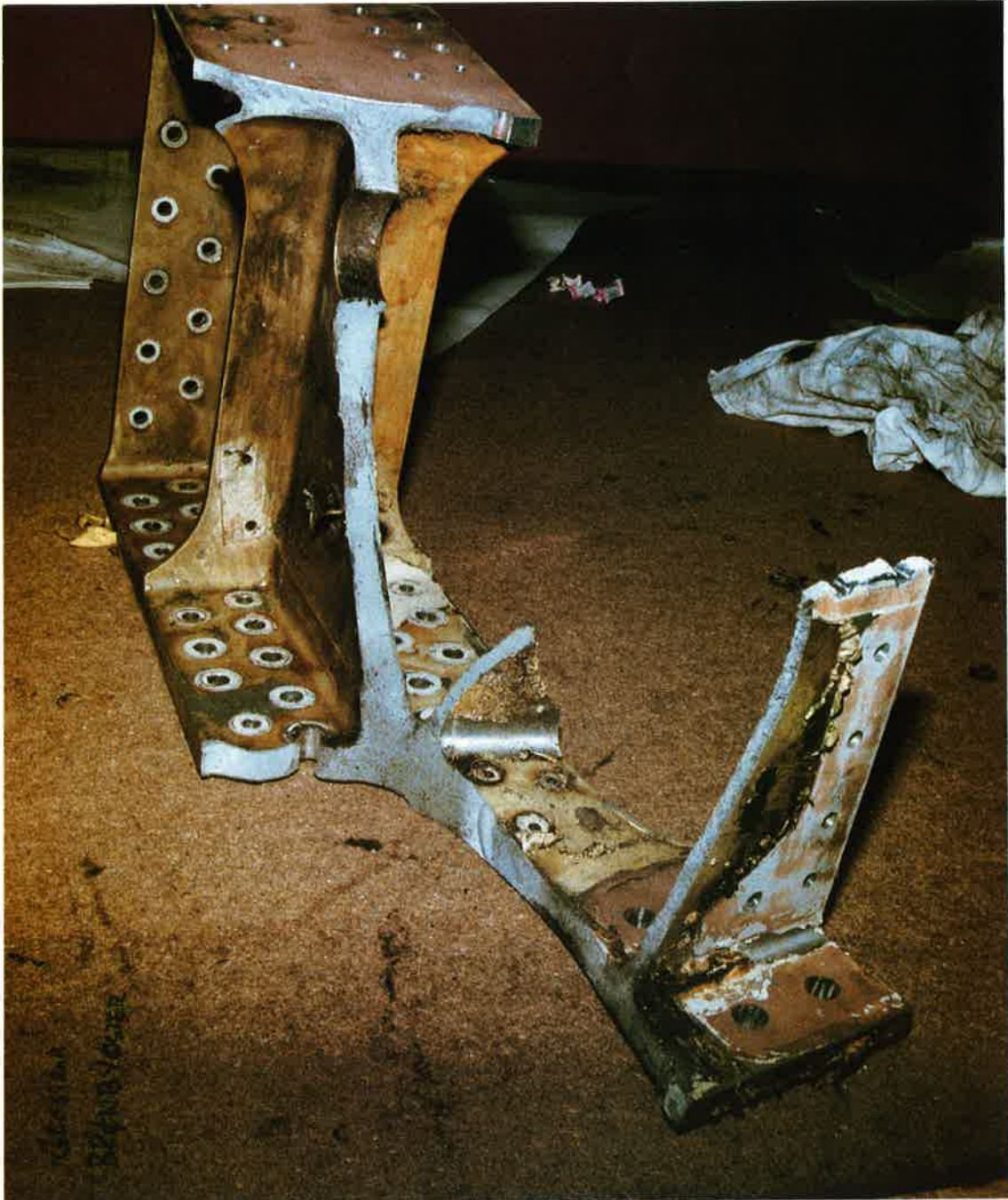
BAC 1-11 FAILED MANACLE BEAM
