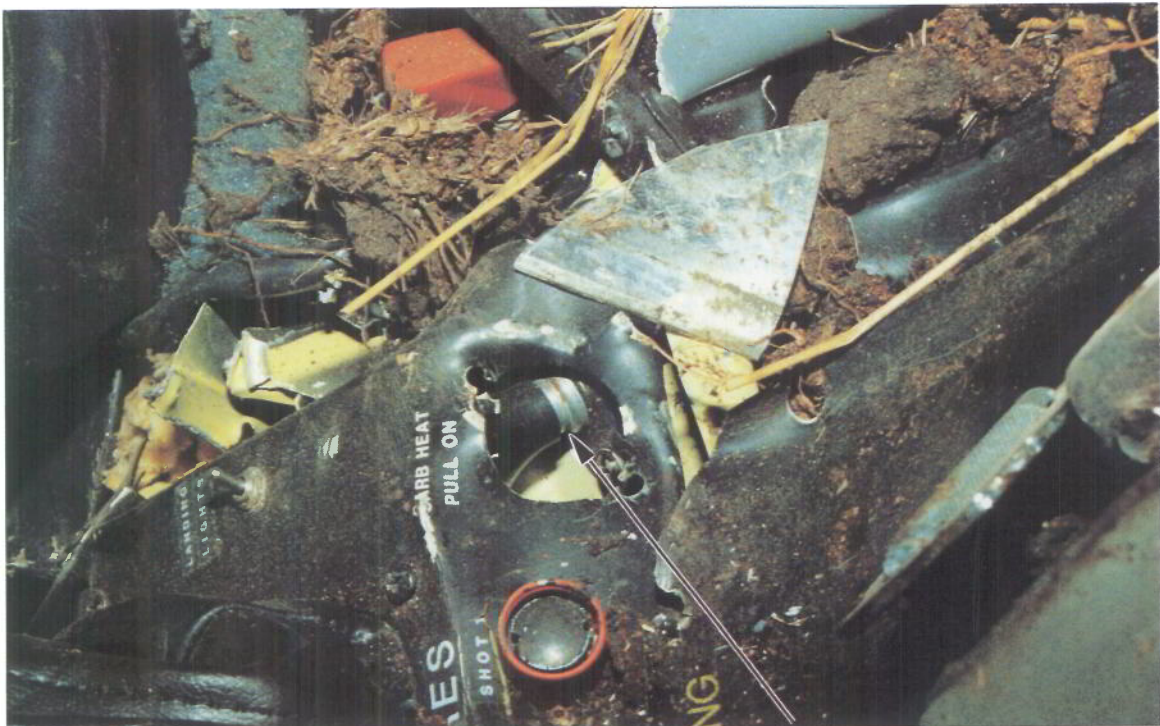
G-BPPC: View of centre console showing carburettor heat control knob fully down (cold position)
