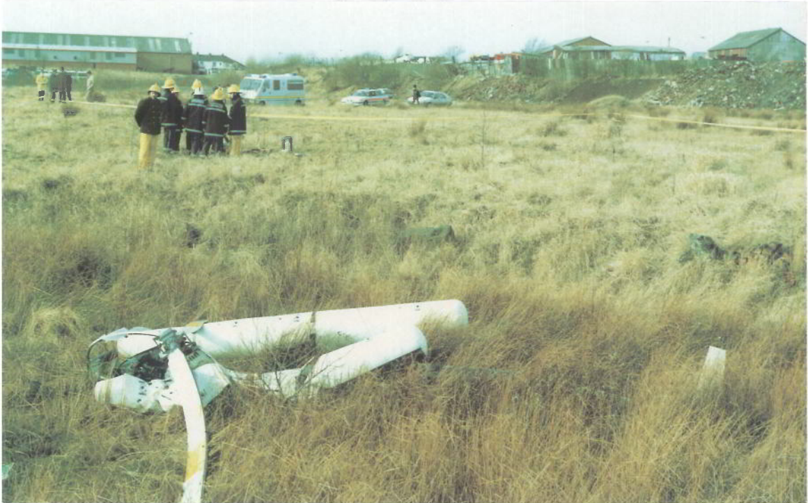
G-BPPC: Note lack of rotational damage to main rotor blades
