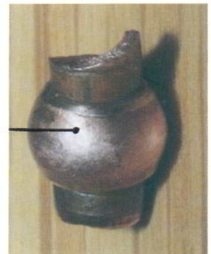
BROKEN PIPE END c.w. OLIVE
