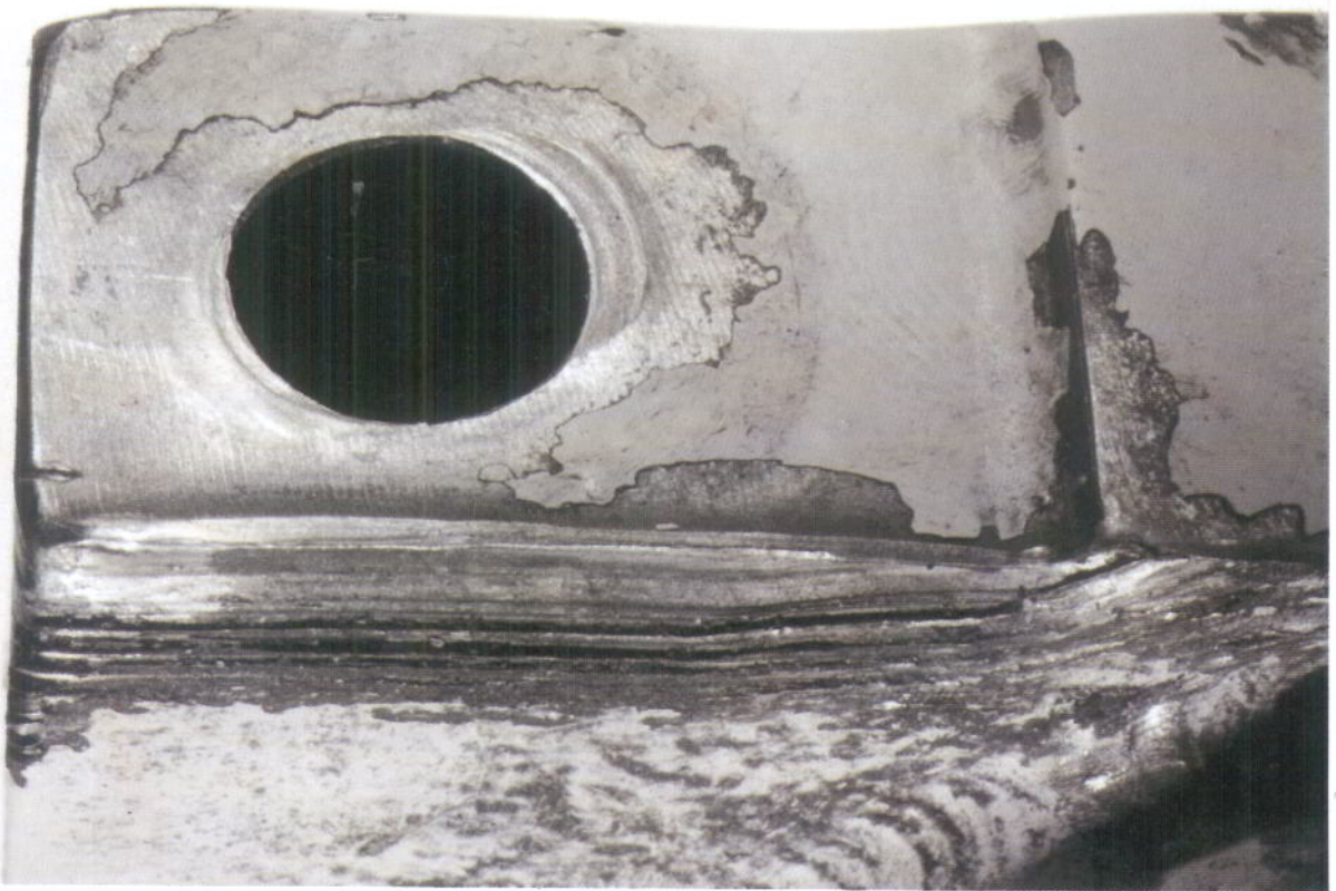
Photograph No. 6. Ovality of the bolt hole in the top of the nose landing gear leg.
