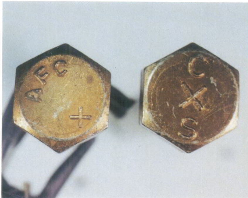
Photograph No. 2. Head of failed bolt (left) & "good" bolt (right).
