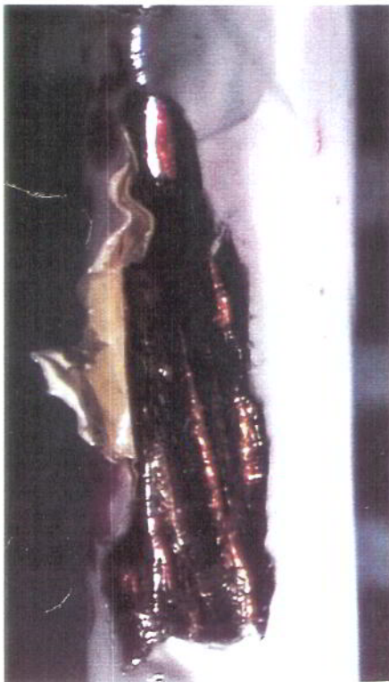
Details of 'cutting/slicing' damage to the outer insulation of two of the wires shown above left, leading to exposure of the polyimide insulation.
