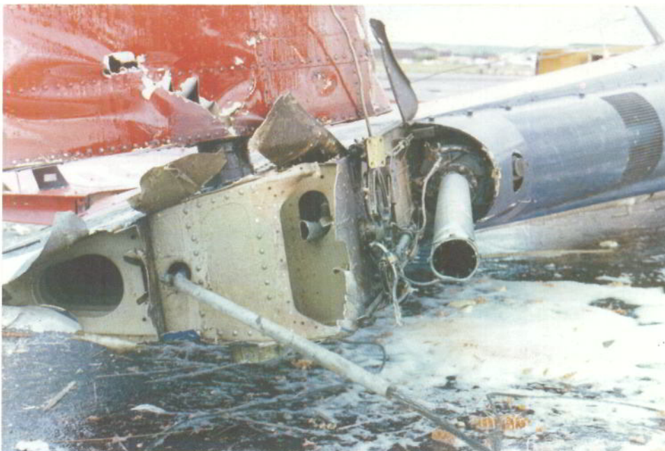
Photograph 3 Top of pylon assembly (Showing detachment of upper pylon and tail rotor driveshaft)
