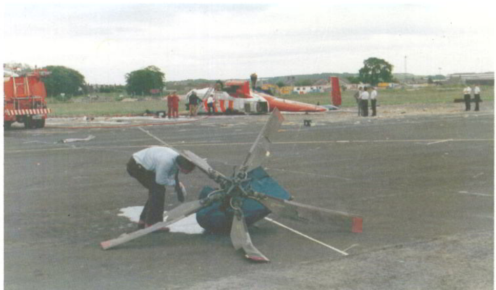
Photograph 2 Tail rotor and gearbox assembly (Note sections missing from trailing edges of blades)
