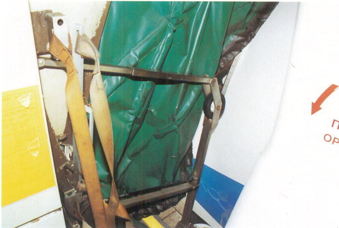
Forwards railing and idler wheel at full extension (not in contact with skin).
