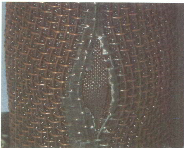
Burst area in oil pressure screen filter
