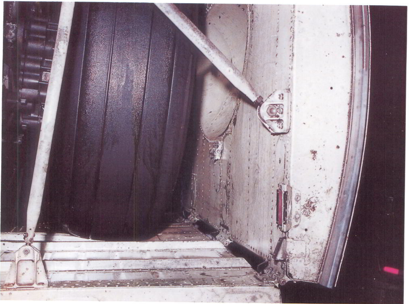
PHOTO 1 NO 7 WHEEL RESTING IN LEFT BODY GEAR DOORS - (Viewed facing rearwards)
