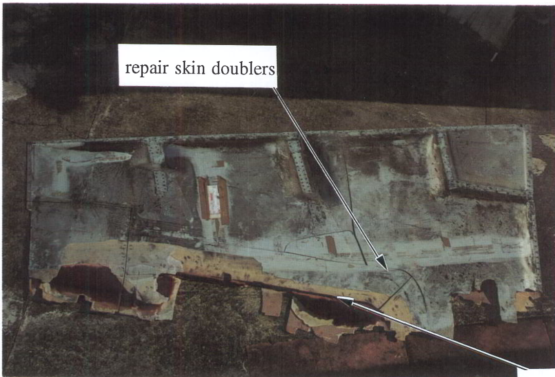
G-BDXH - View of failed wing trailing edge panel showing repaired area
