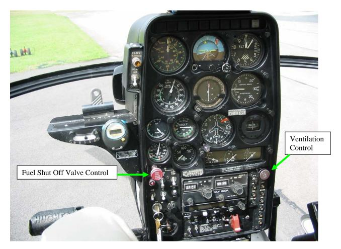
**Figure 4** (Instrument console – Hughes 369HS)
