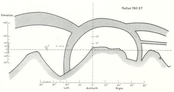
$\times$  Indicates other aircraft's estimated position if overshoot assumed to have occured at 150 feet  $\circ$  Indicates other aircraft's estimated position if overshoot assumed to have occured at 300 feet
