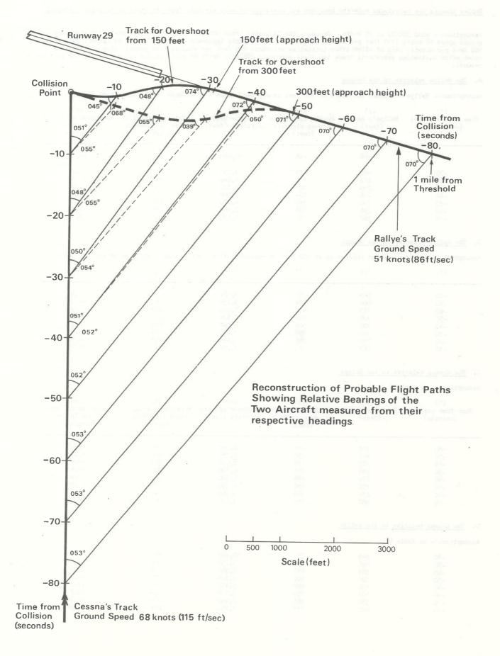
Assumptions:- wind 300(T) at 20 knots. Cessna:- TAS 78 knots; track 000°(T); course 347°(T); drift 13° starboard; ground speed 68 knots (115 feet per second). Rallye:- TAS 70 knots (approach and climb); rate of decsent on approach 500 feet per minute; rate of climb after initiating overshoot 800 feet per minute; five second delay in achieving climb after initiating overshoot; track (on final approach) 286°(T); drift 4° port; ground speed 51 knots (86 feet per second).
