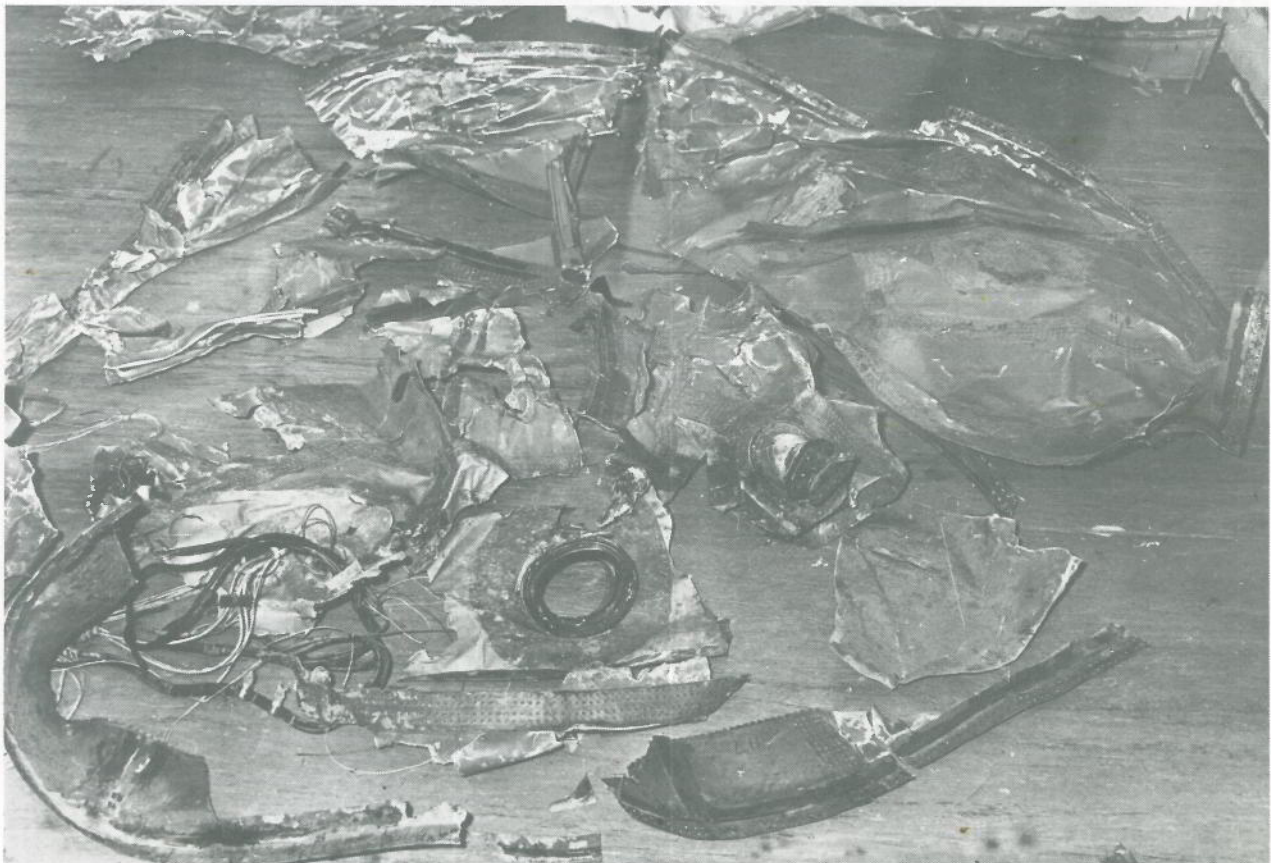
Figure n° 9: Typical "step," marks along tears in the rear pressure bulkhead.
