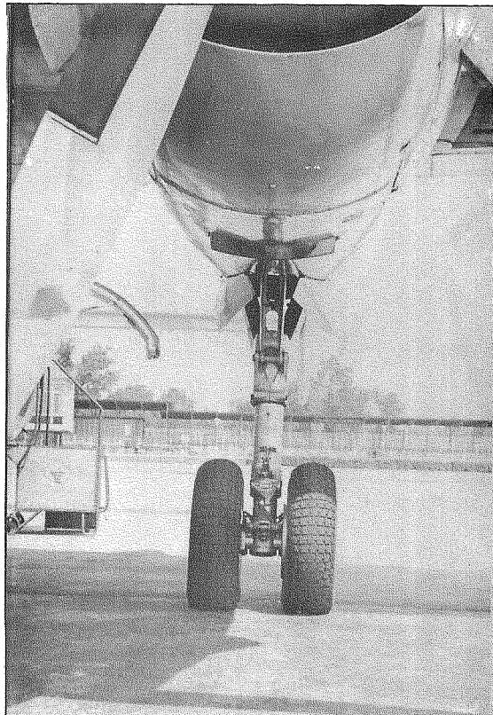
Fig. 13 Front view of main undercarriage.
