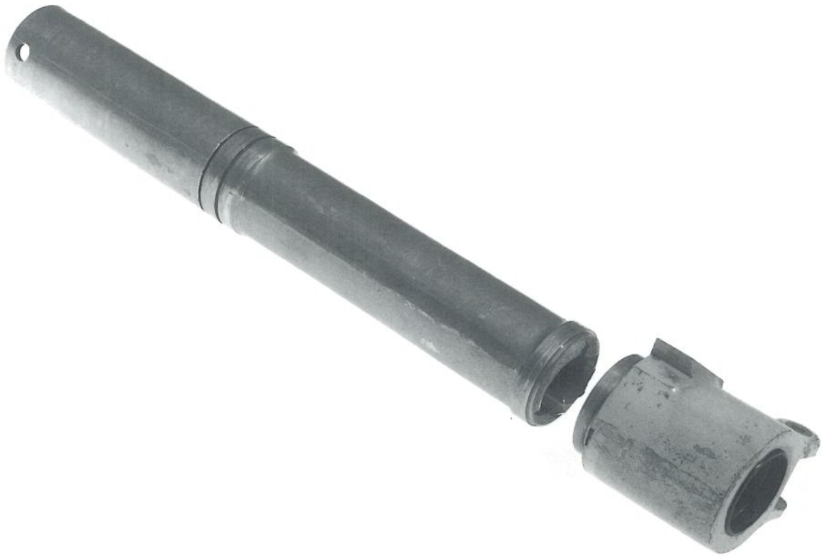
General view of fractured nose leg from G-BSVW
