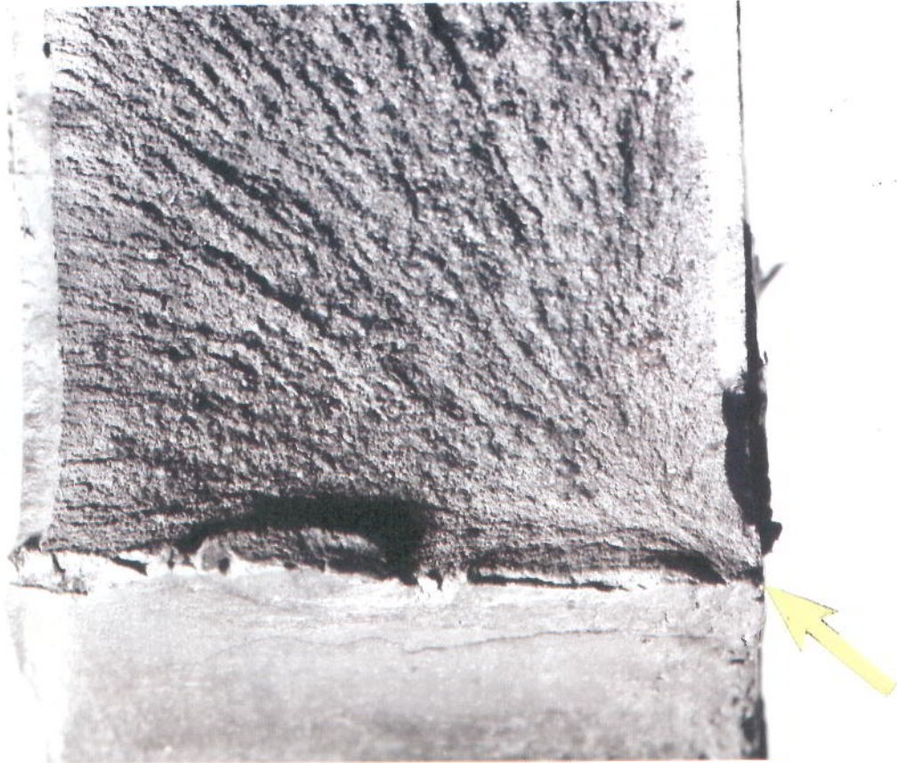
13. Showing fracture surface above outboard bolt hole, with origin arrowed.
