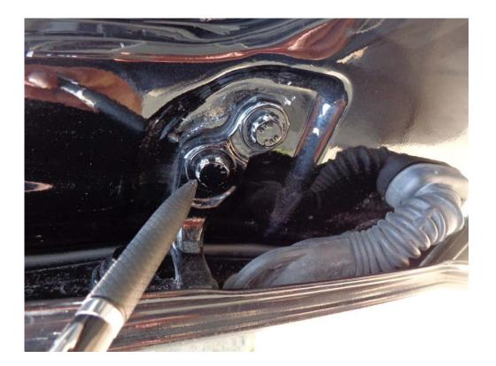
Rounded bolt – Suggesting wrong tool was used in the repair process
